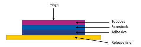
Figure 1 Schematic representation of Pressure Sensitive Labels
